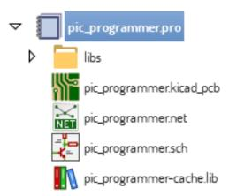
Double-clicking on the schematic file runs the schematic editor, in this case opening the file **pic\_programmer.sch**. Double-clicking on the board file runs the layout editor, in this case opening the file **pic\_programmer.kicad\_pcb**. Right clicking on any of the files in the project tree allows generic file manipulation.
