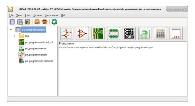
The main KiCad window is composed of a project tree view, a launch pane containing buttons used to run the various software tools, and a message window. The menu and the toolbar can be used to create, read and save project files.
