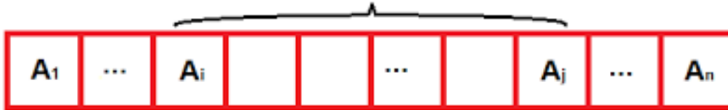
Figure 8: The remaining coins are \{ A_i \dots A_j \} and it is your turn. Let P(i, j) denotes the maximum amount of money you can get. Should you choose A_i or A_j ?
