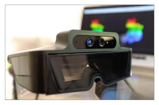
Here is the front view of the Meta 1 Developer Kit, showing the optical see-through stereoscopic 3D display and 3D range-sensing camera (introduced in *Chapter 5*, *Rendering of Point Cloud Data for 3D Range-sensing Cameras*):
