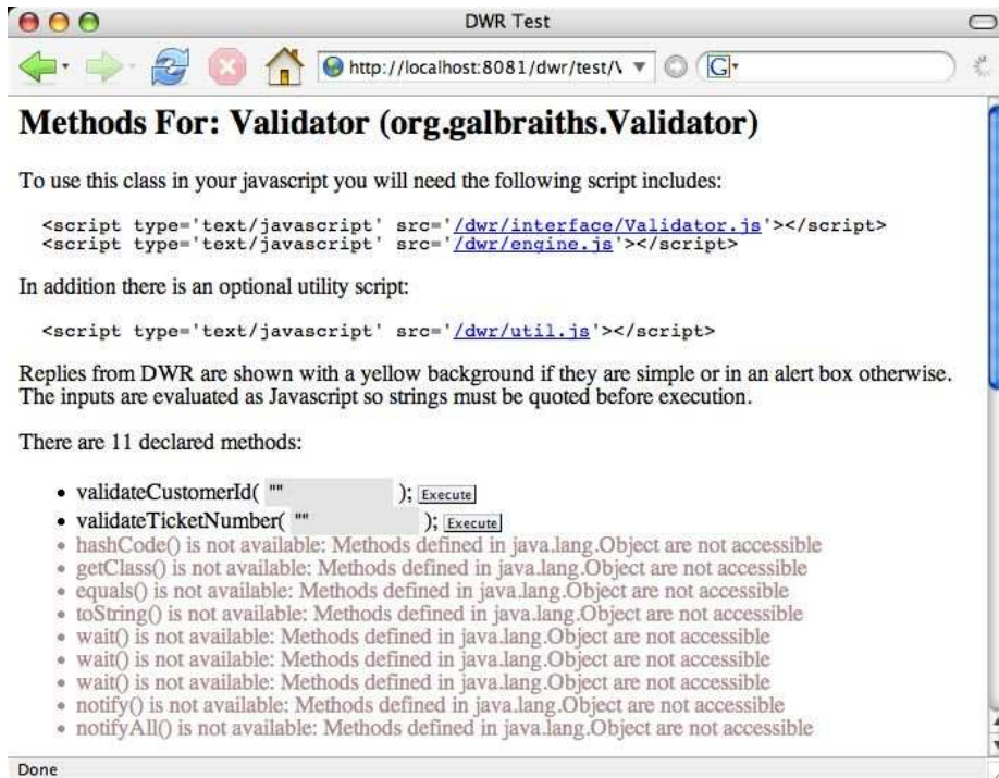
Figure 14.2: DWR Exposing the Validator Class
