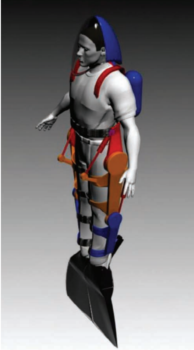
FIGURE 3-1 Example of a swimming exoskeleton. Such an exoskeleton not only has the potential of increasing the speed and range of a swimmer but can also increase stealth by mimicking fishlike rather than machinelike movement. SOURCE: Reprinted with permission from Peter Neuhaus and the Institute for Human and Machine Cognition at the University of West Florida.
