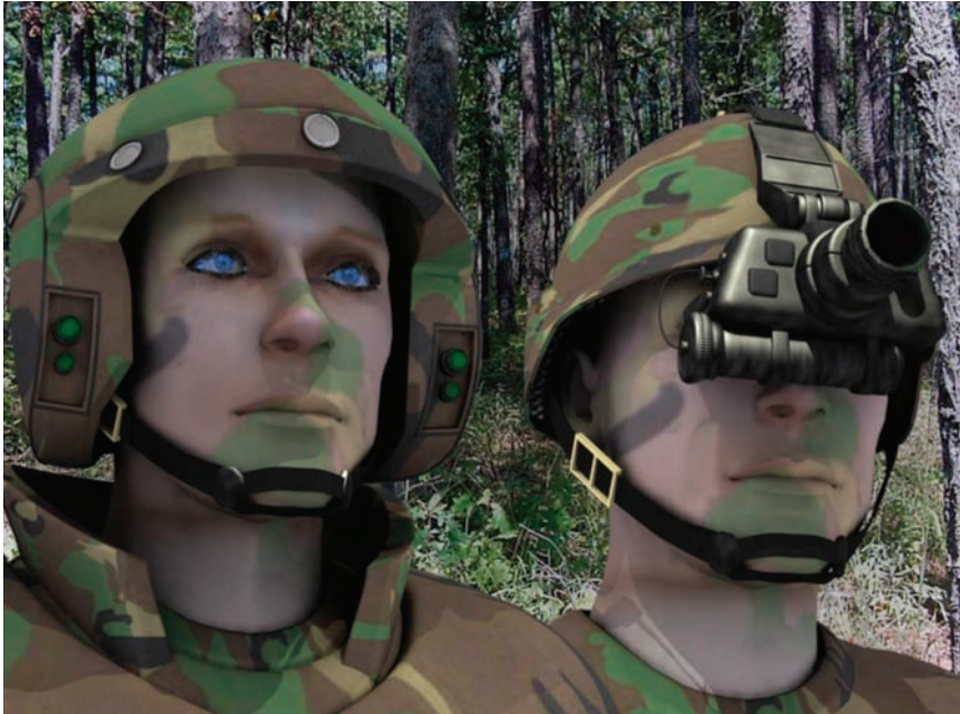
FIGURE 3-3 Visual prosthesis design for combat operations. Unlike current night vision systems (right), sensory substitution for night vision would not impede use of the eyes at night (left). SOURCE: Reprinted with permission from Anil Raj and the Institute for Human and Machine Cognition at the University of West Florida.
