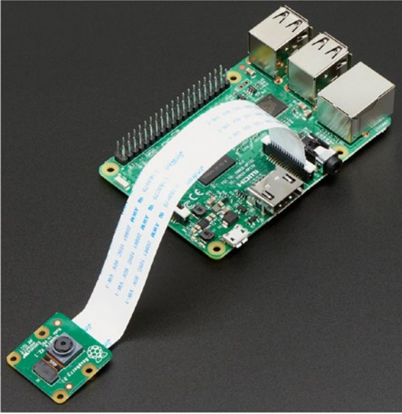
Figure 3-4. Attaching the Pi Camera module to the Pi
