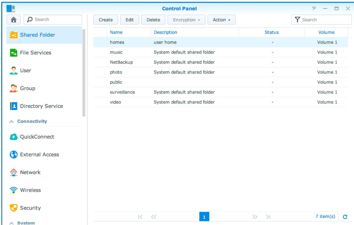
The screenshot shows the Synology Control Panel interface. On the left, there is a sidebar with various management links: Shared Folder (selected), File Services, User, Group, Directory Service, Connectivity (QuickConnect, External Access, Network, Wireless, Security), and System. The main panel is titled "Control Panel" and displays a table of shared folders. The table has columns for Name, Description, Status, and Volume. There are seven items listed:
