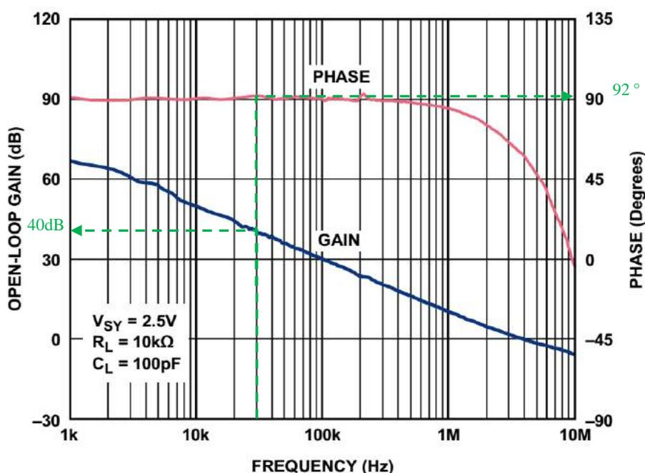
Figure 21. Open-Loop Gain and Phase vs. Frequency
