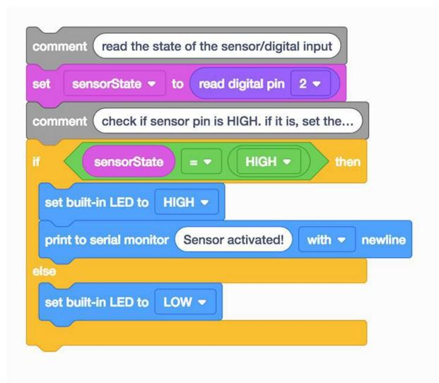
Let's use the Blocks coding interface to listen to the PIR movement sensor, and then make the decision to turn on the LED depending on the sensor state: activated or not activated.
