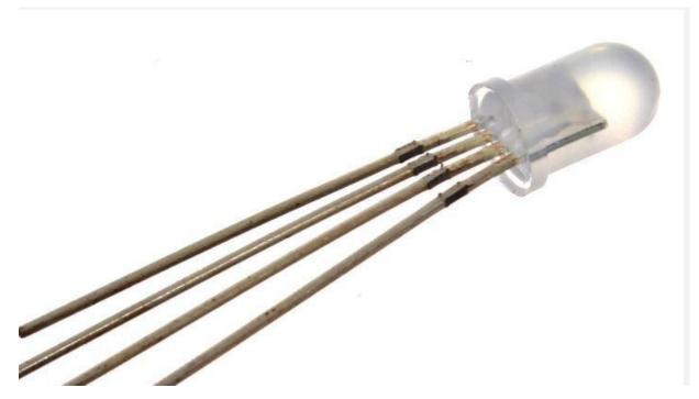
The RGB LED has 4 pins, one for each color (Red, Green, Blue) and a standard cathode. It has color-coded diodes that separate the trees that can be combined to create all kinds of color! Any color is possible depending on how bright each diode is.
