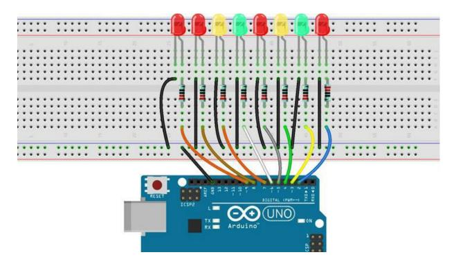
In this study, we will conduct a simple yet fun test - we use LEDs to create flowing LED lights. As the name suggests, these eight consecutive LEDs glow and dim in sequence, like flowing water.
