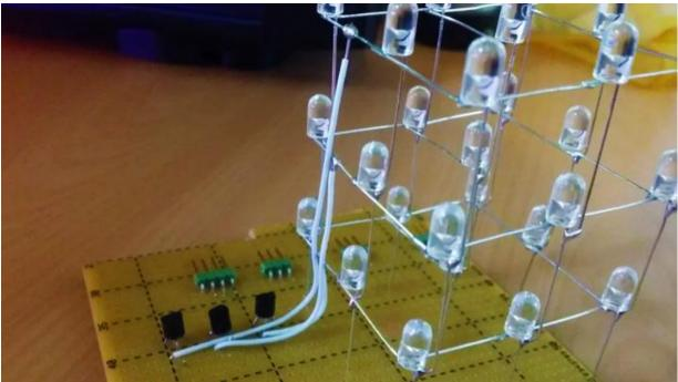
Use 3 wires to connect each layer to one of the transistors. You can see which pin you should be solder to the perfboard structure in step 5.
