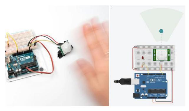
Let's learn to feel the movement in the PIR sensory chamber and Arduino's digital input. We will connect the circuit using a breadboard and use a simple Arduino code to control a single LED. We'll use Tinkercad Circuits to mimic a circuit so you can follow without elements, and show you how to build a visual circuit too.
