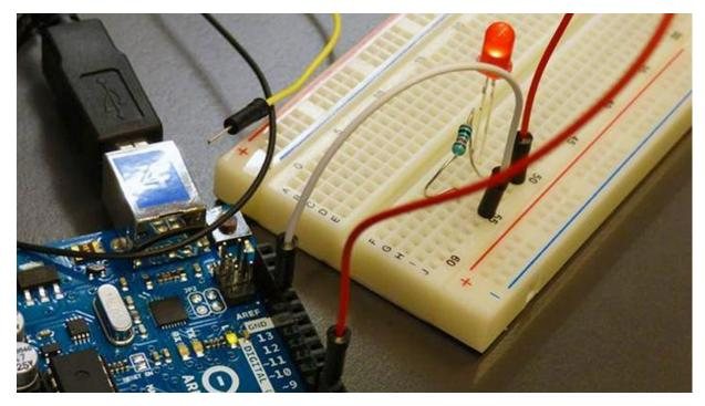
As I explained earlier, current electricity flows from high power to low power. At this stage we will be removing all 5V emissions from Arduino, so for now it will flow from 5V out of Arduino, past our circuit, back to the Arduino "ground" pin. The first thing we will empower is the LED.
