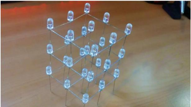
Use something like a soldering hand to solder all the anodes in the anode in the layer below.
