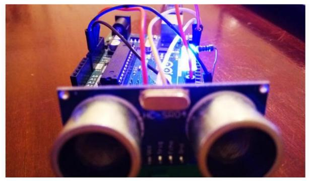
Ultrasonic module from HC - SR04 provides unbalanced measuring function of 2cm - 400cm, accuracy ranging from up to 3mm. Modules include ultrasonic transmission equipment, receiver and control circuit.
