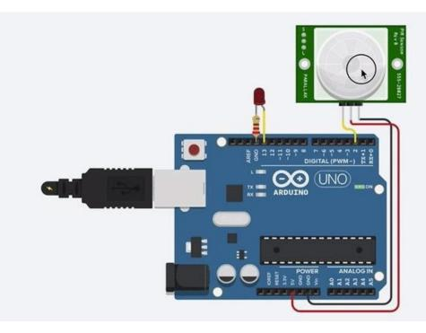
Check the circuit sample here in the embedded circuit below by starting the simulation and clicking the circular motion sensor. This will activate the highlighted area in front of the sensor with the "object" circle inside. You may need to expand the view when the circle is closed on the screen. Click and drag the "object" circle before the sensor to represent the movement. The LED will turn on for a moment when motion is detected.
