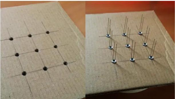
To start we have to make 3 layers of 3x3 LED; s. An easy way to do this is to get a piece of cardboard and draw holes with a 3x3 pattern. Make sure the LEDs will not come in when you press them in the holes. In the end it should look like a picture.
