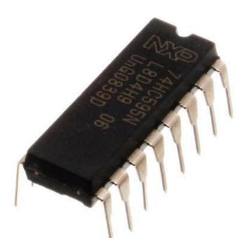
Next we will look at a data sheet 595 to find the appropriate connecting pins for them. The first image above shows 595 pin connections. There are 16 pins in 595, with a 1-16 label. Note the half-marking on one side of the chip, the # 1 pin is always located on the left side of the chip. All pins are numbered around the chip to the opposite side of the clock.
