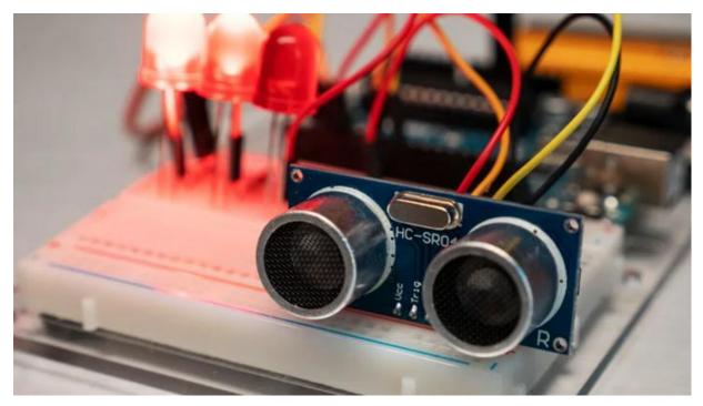
If you are creating a visual version of this region, you can try it with a serial monitor for Arduino software (magnifying the glass button at the top right of the sketch window), activating the sensor with your hand, body, notebook, etc.
