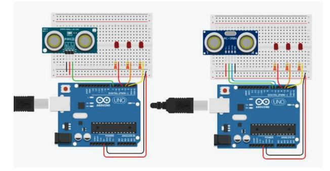
As you learned from the introduction, first connect your Arduino wires to the bread board with power and ground near the circuit
