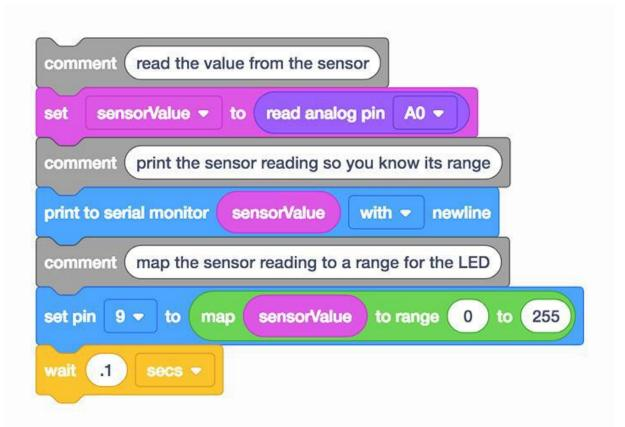
Let's use the code block editor to listen to the position of the photoresistor, and then set the LED to the relative light depending on how much light the sensor sees. You may wish to refresh your memory of the LED analog output in the Fading LED lesson.
