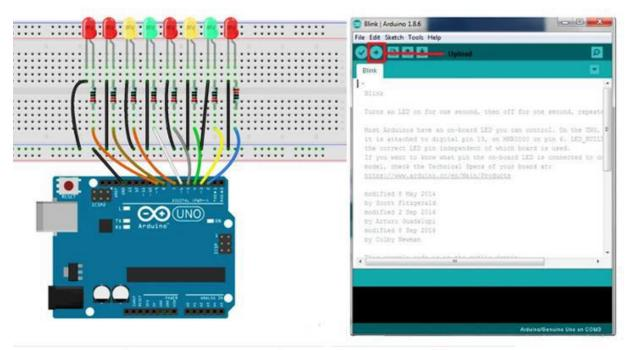
The goal of this experiment is simply to turn on eight LEDs in a row. Eight LEDs are connected to a 2-pin 9 pin respectively. Set them as high quality and the corresponding LED on the pins will light up. Control each LED light time and you will see flowing LED lights.
