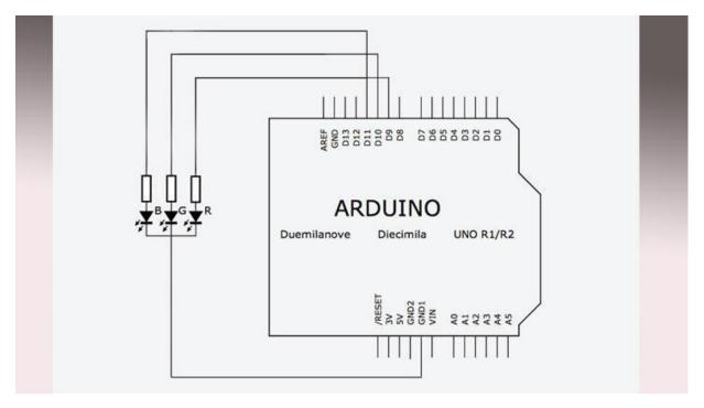
RGB LEDs are really fun, as you can see in the first picture above, each RGB LED is actually made up of three LEDs: one red, one green, and one blue. When you turn on a few LEDs at the same time they will combine to form new colors.
