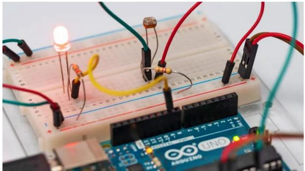
Let's learn how to read photoresistor, a light-sensitive type of flexible resistor, using Arduino Analog input. Also called LDR (light-based antagonist).
