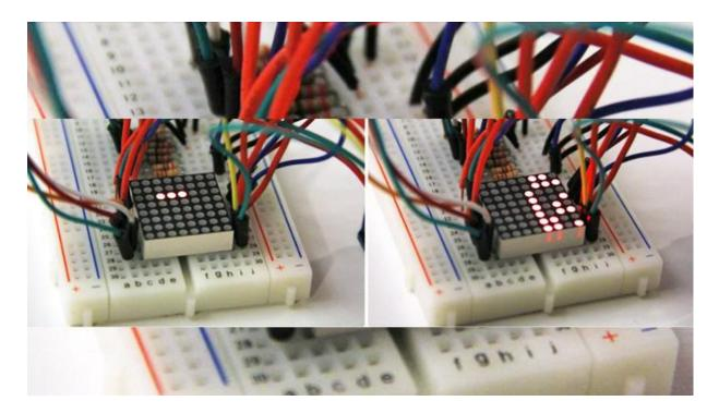
So far the code we used to send data to LED is hard to write. Includes explicit allocation of HIGH or LOW status to each Arduino pin connected to the column. If we wanted to edit the matrix to show a different pattern for each of the 8 lines, we would have to write a line of multiple code. Here's how to put things together:
