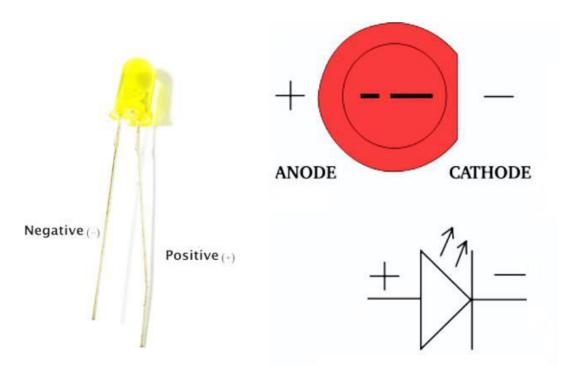
Light Emitting Diode or LED is basically a Diode that can emit light.
