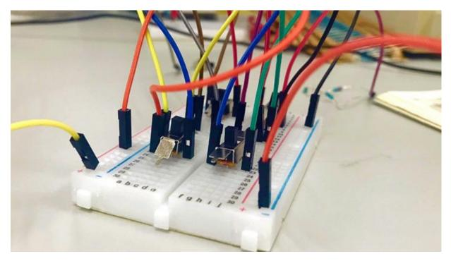
Bread boards should make temporary electrical connections between objects so that we can inspect the circuits before fully assembling them permanently. The whole class will be held on the bread board so we can reuse items and make quick changes to the circuit. Bread boards have holes in which you can insert wires or other electrical appliances. Some of these holes are electrically connected to each other by means of metal straps under the bread board. Here's how communication works:
