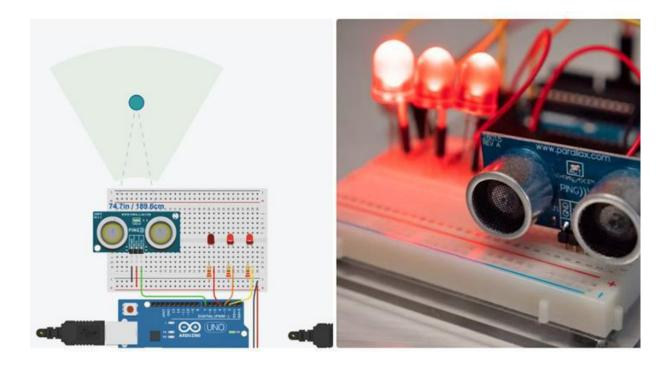
Let's measure distances with an ultrasonic rangefinder (sensor distance) and Arduino's digital input. We will connect the circuit using a breadboard and use a simple Arduino code to control a single LED.
