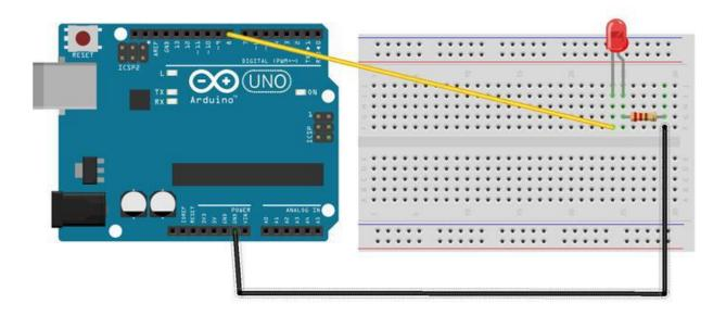
So far we have been using the delay function () to pause the Arduino drawing so that the time interval between the two Arduino commands passes. In the LED blink panel, we used the delay to set the Arduino turn on and off:
