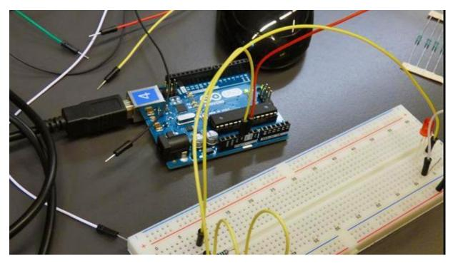
Arduino is a pocket-sized computer (also called a "microcontroller") that you can use to control circuits. Works with a foreign name through sensors, lead, engines, speakers ... even the internet; this makes it a flexible platform for many creative projects. Other popular uses include:
