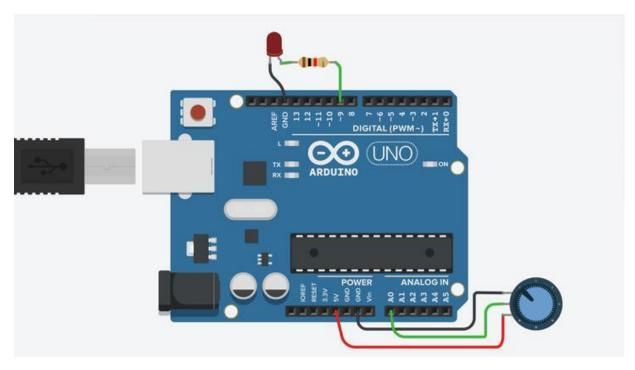
analogRead (pinNumber) - analogRead () read from one of the Arduino analog pins and output a value between 0 (voltage per pin = 0V) and 1023 (voltage per pin = 5V), if the analog pin voltage was 2.5V, then it would print:
