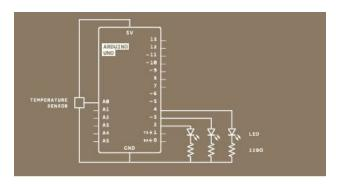
Now, you are doing it manually, but you can achieve that by calibration. You can use the button to define the reference temperature, or let the Arduino pick a sample before a loop() starts and have it as the point of reference.
