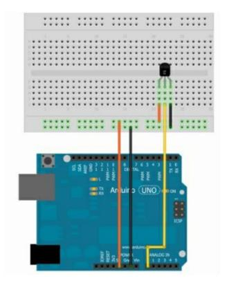
Example 7: Temperature sensor with serial interface (Coding)
