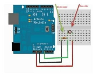
Example 8: Showing the strength of the LED light on the serial monitor (Coding)
