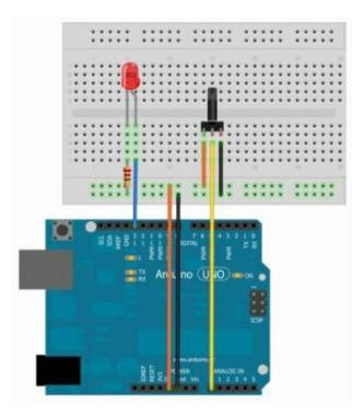
Example 4: Control light amount using potentiometer (Coding) //create new file form the Arduino IDE and write the following code: const int sensorPin = A0; const int LedPin = 13; int sensorValue; void setup () { PinMode (LedPin, OUTPUT); }
