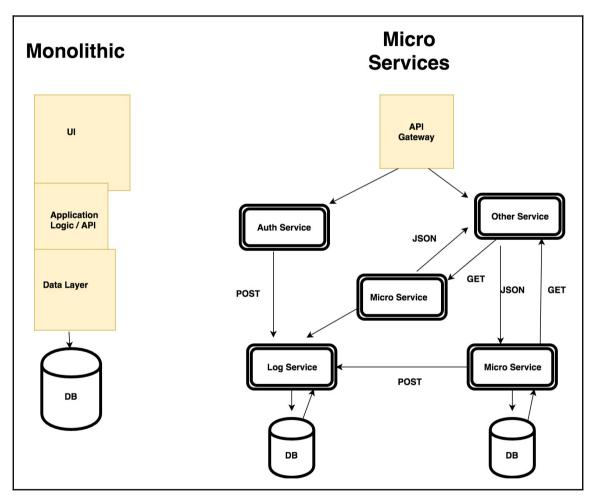
This diagram depicts the structure of monolith and microservice architectures. A monolith has everything wrapped in the form of an onion. It is called a tightly coupled system. In contrast, microservices are individual, easy to replace and modify. Each microservice can talk to each other through various transport mechanisms, such as HTTP and RPC. The format could be either JSON or Protocol Buffers.
