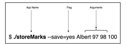
Suppose that we have a command-line app called storeMarks for saving the marks of a student. It has a flag (called save) to specify whether details should be pushed to DB or not. The arguments that are given are the name and actual marks of the student. We already saw how to collect the flag values in the program. In this section, we will see how to collect program arguments in an expressive way.
