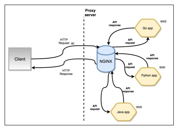
If you see, the illustration client is talking directly to Nginx instead of the ports where other applications are running. In the diagram, Go is running on port 8000 and other applications are running on different ports. It means the different servers are providing different API endpoints. If the client wishes to call those APIs, it needs to access three ports. Instead, if we have Nginx, it can act as a proxy server for all three and simplifies the client request-response cycle.
