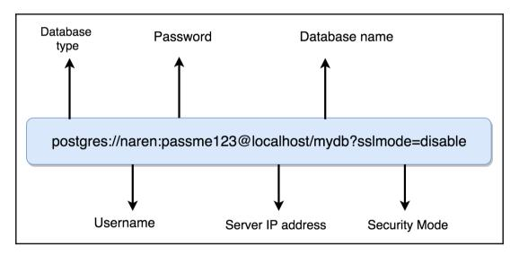
The connection string should consist of the database type, the username:password pair, the database server IP, and the sslmode settings. We are then creating a table called web\_url. All the error handlers are there to specify if something goes wrong. The InitDB function returns the database connection object to whatever program imports the function. Let us write the main program to use this package:
