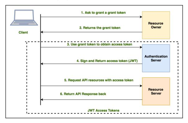
In this diagram, we can implement the dashed section using JWT. Authentication is happening at the authentication server level and authorization happens at the resource server level.
