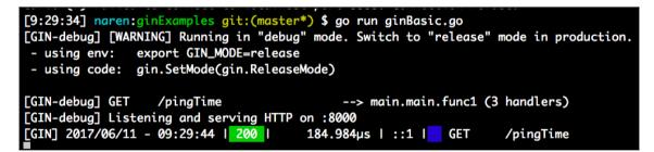
It is Apache-style debug logging showing the endpoint, the latency of the request, and the REST method.
