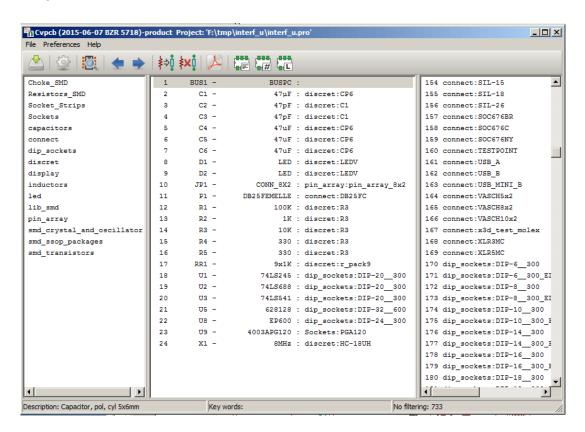
Filtered by list of footprint filters assigned to the selected component. The component filters are listed on the center pane of the status bar at the bottom of the main window.
