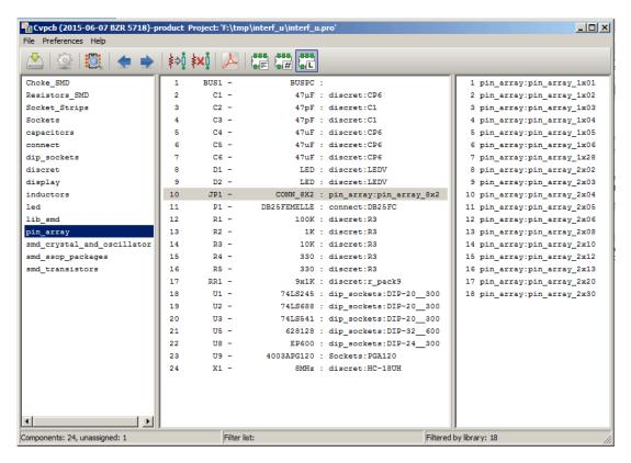
The filtering can be combined to form more complex filtering to help reduce the number of footprints in the footprint pane.
