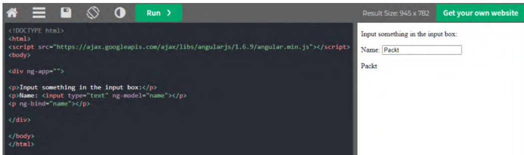
Figure 5.5 – Basic AngularJS web application code snippet (source: https://www.w3schools.com/angular/tryit.asp?filename=try_ng_intro )
